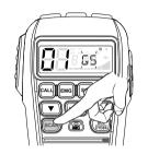
If the Priority Channel becomes active the radio will stay on that channel for as long as the signal is present. If the received signal ceases, Priority Scanning continues after 3 seconds.
